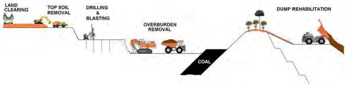
Gambar 4.3 Proses Bisnis Land Clearing, Drilling & Blasting, Overburden Removal dan Rehabilitasi
